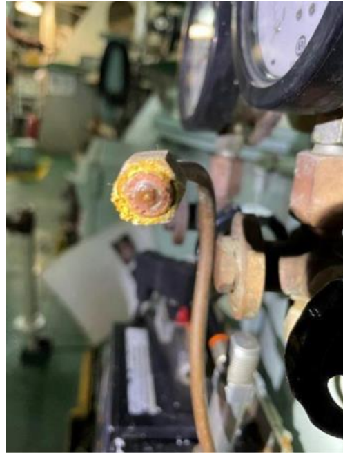
Figure 3 – another view of a blocked 15ppm bilge alarm sample line outlet with no flow.
