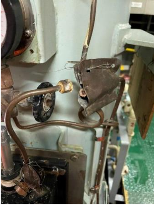
Figure 2 - a blocked 15ppm bilge alarm sample line outlet with no flow.
