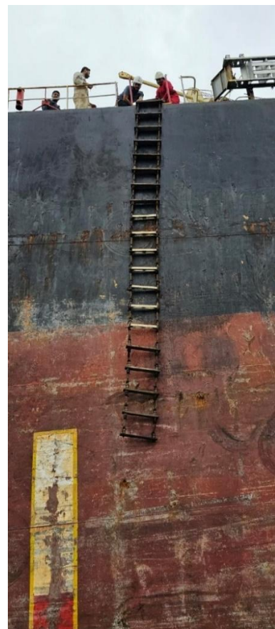
Figure 4. Incorrect ladder used, no spreaders, and combination arrangement not provided for safe embarkation to the vessel despite freeboard of vessel more than 9 m.
