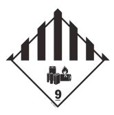
For those shipments exempted by SP188, every package must show the lithium and sodium ion battery as per 5.2.1.10 and illustrated by the example below:
