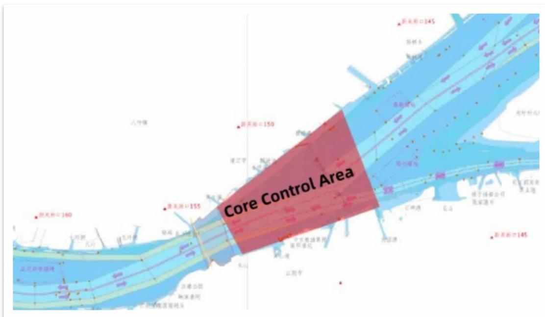
(1) **Restricted ship speed.** Ship's speed in the core control area shall maintain at 6-10 knots.
