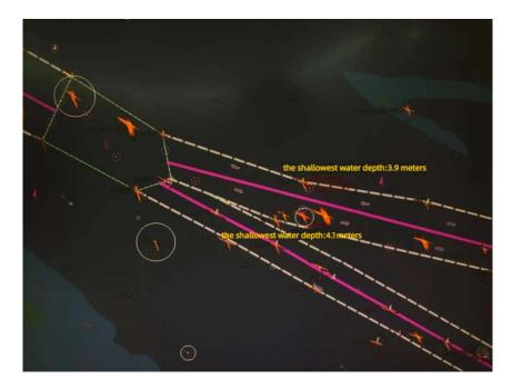
Vessels sailing through the Jiuduansha Precautionary Area to the South Channel Pilot Waters in strong wind and waves condition, shall pay attention to the water depth changes near the channel boundary.
