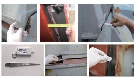
Photograph 3 Using feeler gauges, yardsticks and depth gauges during an inspection
