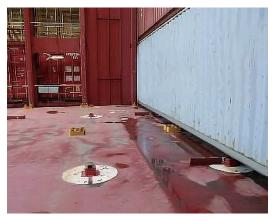
Photograph 22 Pontoon covers on container vessel properly marked/indicated
