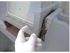
Photograph 14 Measuring clearance of locator with tapered feeler gauge.
