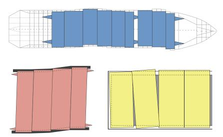
Figure.1 Illustrating relative movements between panels. (Courtesy MacGregor)
