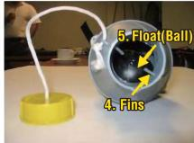
Photograph 19 Drain systems: Principle - non-return valve
