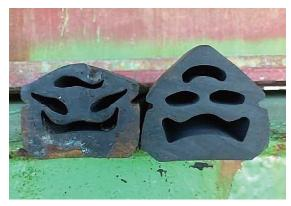
Photograph 9 Overcompressed CAT seal
