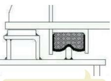
Figure 4 Bearing pad wear will result in overcompression of the packing rubber.
