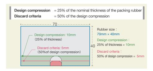
So for a 70x40mm packing rubber with a design compression of 10mm, 5mm of permanent set will be the limit for replacement. In case of the normal type of CAT seal, a round shaped profile, instead of the triangular one, indicates that the packing rubber is nearing the end of its in-service life.
