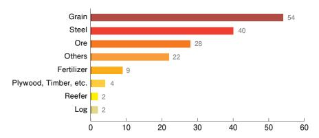
Graph 1 Number of Sea Water Damage on Bulk Carrier, General Cargo Vessel 2016PY-2020PY
