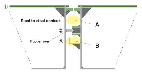
Figure.2 Showing the 3 safety barriers in hatch cover design, i.e. the steel hatch plating 1, the sealing system 2 and the drain channel 3
