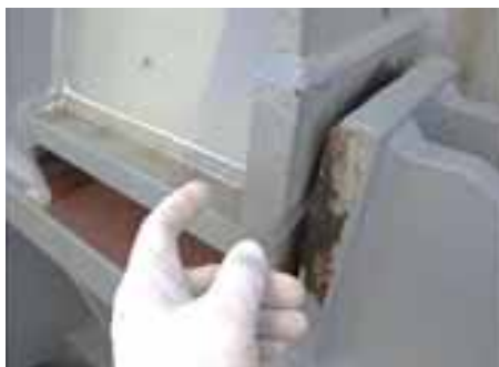
Photograph 14 Measuring clearance of locator with tapered feeler gauge.
