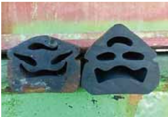
Photograph 9 Overcompressed CAT seal
