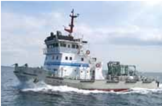
Photograph 27: Water Surface Cleaning and Oil Recovery Vessel, Beikurin (Bay-clean) From the website of the Chiba Port Office, Regional Development Bureau, Ministry of Land, Infrastructure, Transport and Tourism
