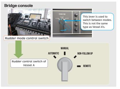
Fig. 42 Steering operation settings Rudder control switch
