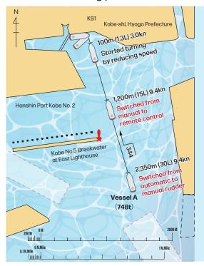
• After passing breakwater No.5 (approximately 1,200m from the quay), the VecTwin system manual control is switched to remote before making a final approach whilst also reducing speed.
