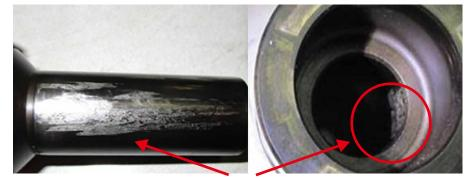
Photograph 5-14 Scratches on the fuel injection valve
