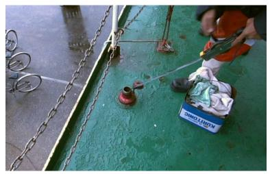
Photograph 4-2(a) Bunkering work: Sounding tank level
