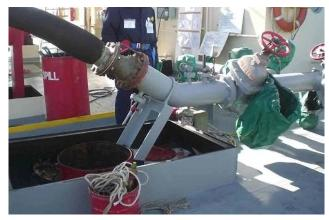
Photograph 5-33(a) Ship bunker manifold
