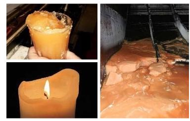
Photograph 5-22 Wax crystal formation in the fuel oil tank
