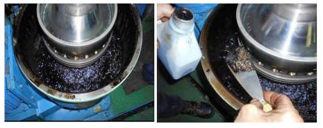
Photograph 5-9 Sludge deposition and precipitation within the rotating bowl of the oil purifier
