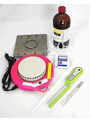
Photograph 5-34 Spot test kit for FO compatibility and stability
