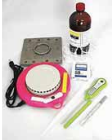
Photograph 5-34 Spot test kit for FO compatibility and stability
