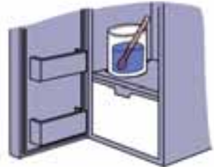
Figure 5-36 Simplified test methods for Pour point in refrigerator
