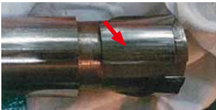
Photograph 5-13 Abnormal wear of plunger and barrel in the fuel injection pump
