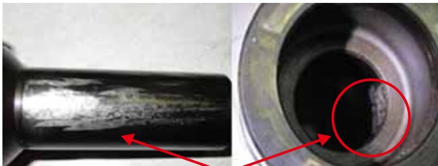
Photograph 5-14 Scratches on the fuel injection valve
