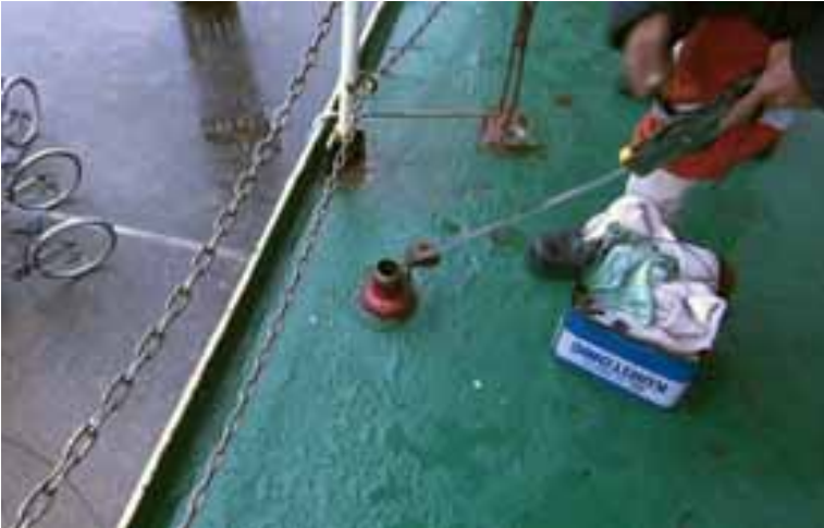
Photograph 4-2(a) Bunkering work: Sounding tank level
