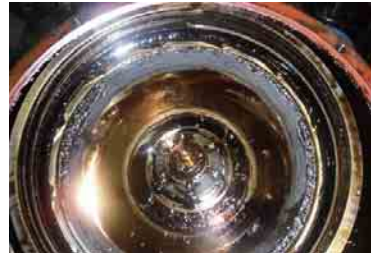
HFO separator : completely blocked by heavy, hard sludge
