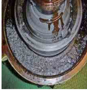
HFO separator after one hour of operation : blocked by heavy, hard sludge
