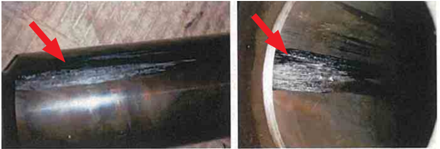
Photograph 5-12 Scratches on the plunger and barrel of the fuel injection pump
