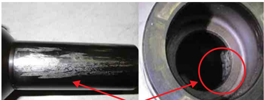
Photograph 5-14 Scratches on the fuel injection valve
