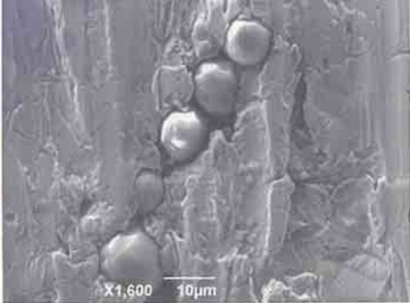
(b) Cat-fines embedded in the piston ring
