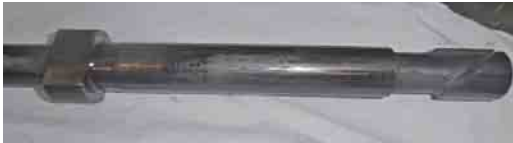
Fuel injection pump : the plunger was found completely seized in the barrel
