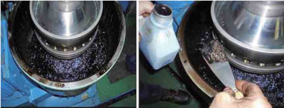
Photograph 5-9 Sludge deposition and precipitation within the rotating bowl of the oil purifier
