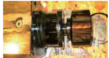
Fuel booster plunger stuck in the barrel
