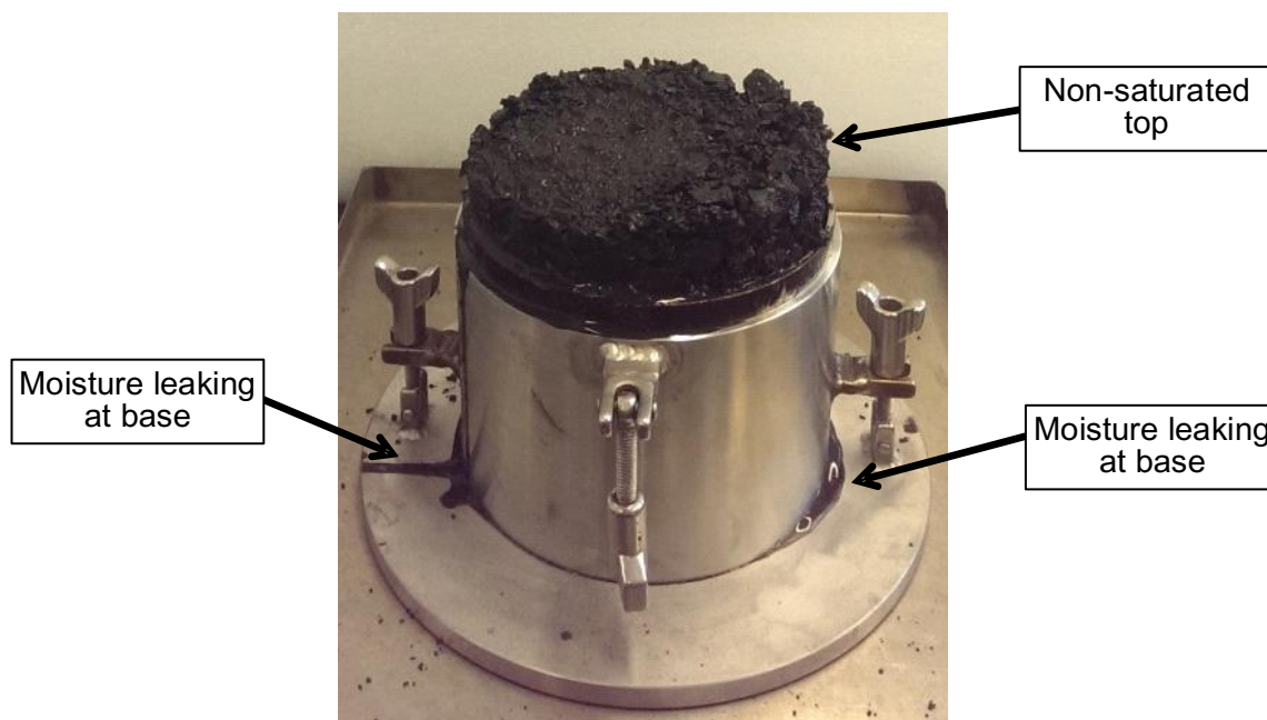
Figure 1.5.5.3.4.2 – Test showing water leakage from the base of the cylindrical mould indicating moisture migration
