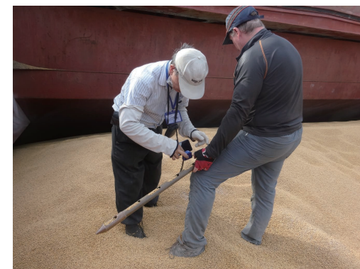
Sampling soybeans with spear
