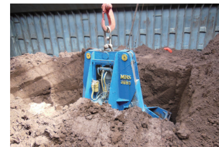
Sampling bauxite in ship's hold by grab
