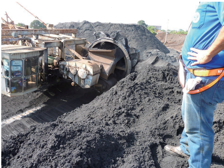
Reclaimer loading iron ore from a stockpile
