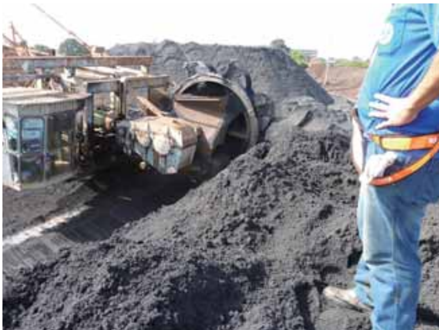
Reclaimer loading iron ore from a stockpile
