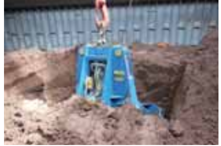
Sampling bauxite in ship's hold by grab
