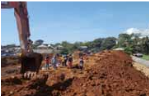
Sampling nickel ore by excavator
