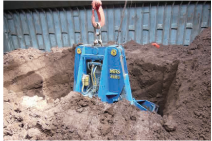
Sampling bauxite in ship's hold by grab
