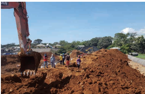
Sampling nickel ore by excavator
