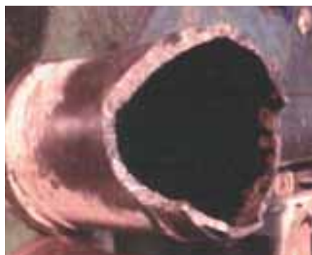
Reference Picture 35 Broken damaged cylinder liner
