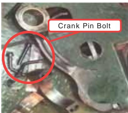
Reference Picture 34 Bending loss of connecting rod
