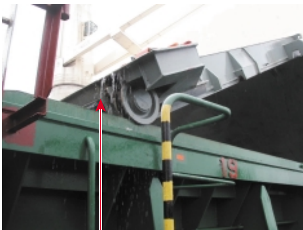
ハッチカバー開放時に流れ落ちる雨水 Showing rain water flows at the time of hatch cover opening.
