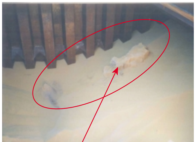
船首部コーミング直下で壁・柱状になった損傷貨物 Showing damaged cargo just under the fore hatch coaming plate, pillar and wall shape.
