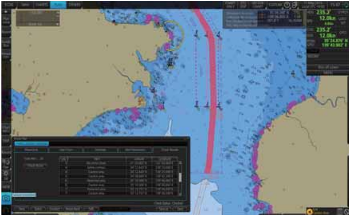
Ref. 4 Sample Display of Safety Check under Voyage Planning (Red Color route : Voyage Planning Route pass through Warning area (special condition area))
