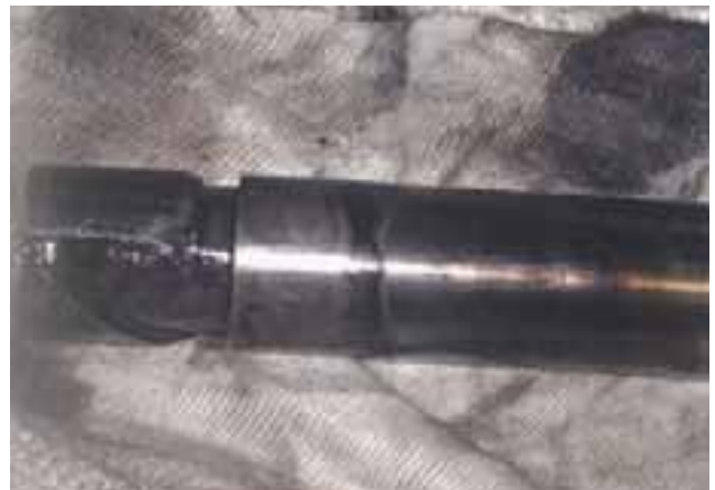
f) Wornout plunger Damage leading to speed reduction in fiscal year 2012 / reference*9
