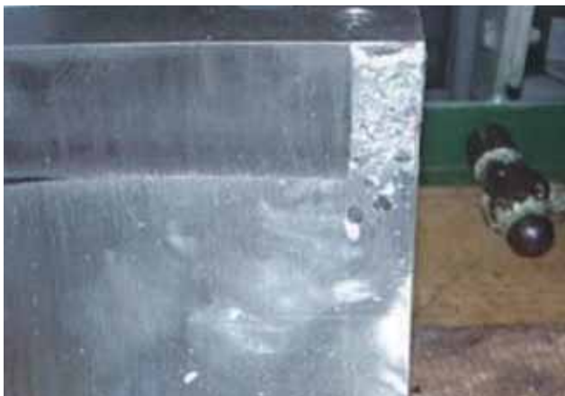
c) Burn-out Intermediate shaft bearing metal(Over heated) Damage leading to speed reduction in fiscal year 2012 / reference*9
