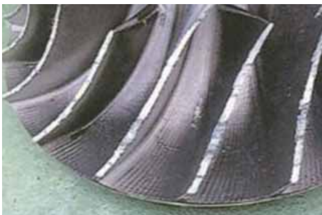
e) Scratch of impeller due to contact with casing Damage leading to speed reduction in fiscal year 2013 / reference *8
