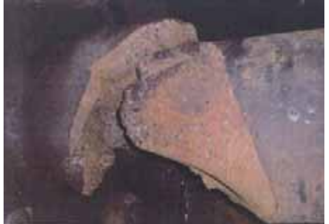
b) Broken intermediate shaft Damage requiring towing in fiscal year 2012 / reference*9
