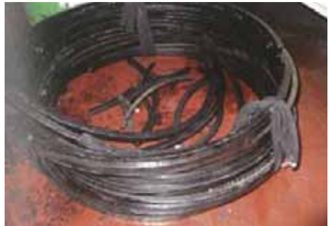
d) Broken piston ring Damage requiring towing in fiscal year 2013 / reference*8
