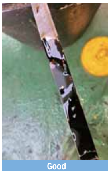
Figure 81 [Normal status] No bubbles on the tape (beautiful glossy reflection)/ reference *19
