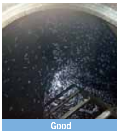
Figure 79 [Normal condition] 6 hours after bunkering: without bubbles / reference*19
