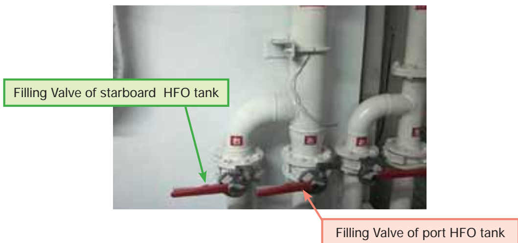
Figure 70 Arrangement of filling valve of HFO tanks for Bunkering (Attention, Filling valve of starboard tank is located on the left side!)
