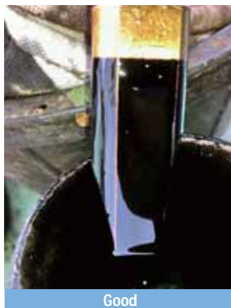
Figure 83 [Normal status] No bubbles on the tape's dip weight (clean glossy reflection) / reference*19
