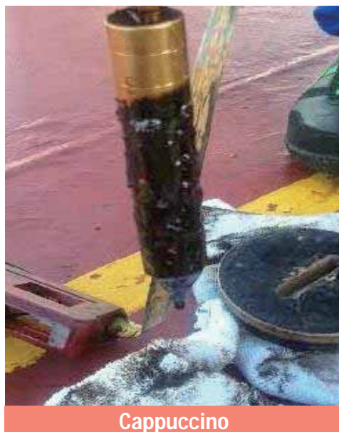
Figure 82 [Cappuccino status] a lot of bubbles on the tape's dip weight (without lustre) / reference*19
