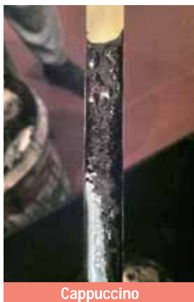
Figure 80 [Cappuccino status] a lot of bubbles on the tape (without lustre) / reference*19
