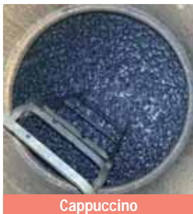
Figure 78 [Cappuccino condition] 2 hours after bunkering: a lot of strong bubbles / reference*19
