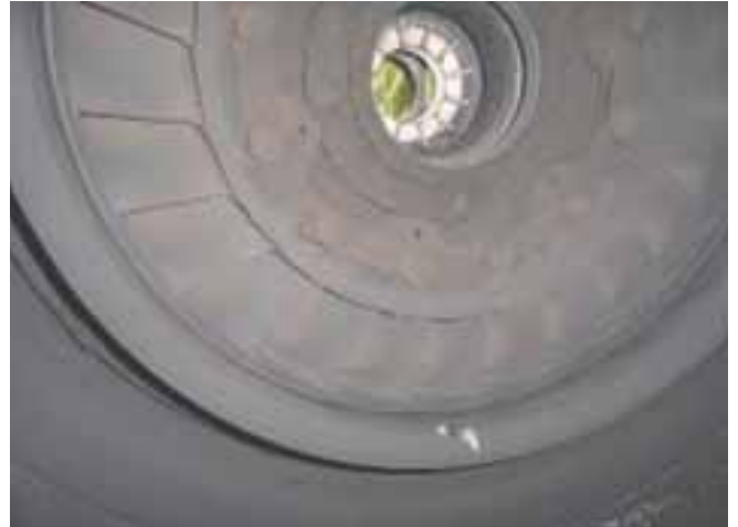
Figure 18 Excessively deformed nozzle ring / reference*7
