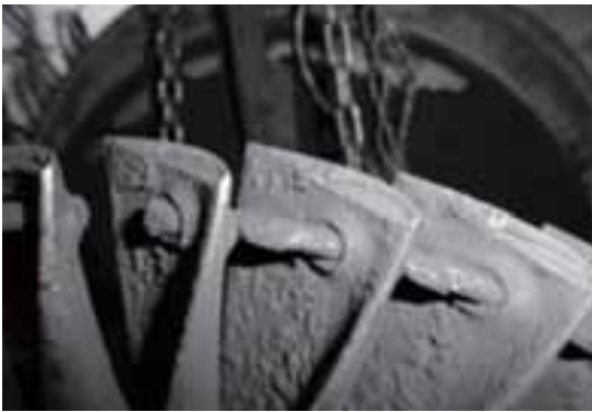
Figure 20 Carbon adhering excessively on turbine blade / reference *7
