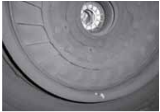
Figure 21 Carbon adhering excessively on nozzle ring / reference*7
