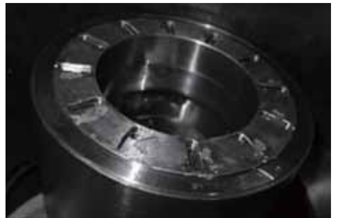
Figure 19 Thrust bearing with metal peeled o / reference*7
