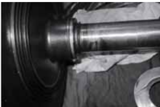
Figure 22 Scratches in rotor shaft / reference*7
