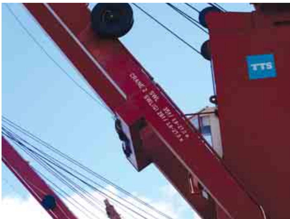
Photo 8 The plate on the side of the jib shows a SWL for hook work of 35 tonnes and a SWL for grab work of 28 tonnes.
