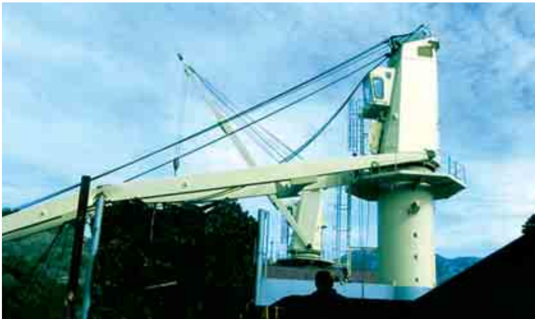
Photo 6 The jib of this crane collapsed and suffered extensive damage as a result of a mechanical failure
