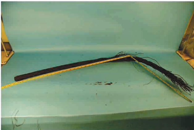
Photo 7 These wires failed when overloaded
