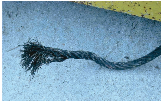
Photo 7 These wires failed when overloaded
