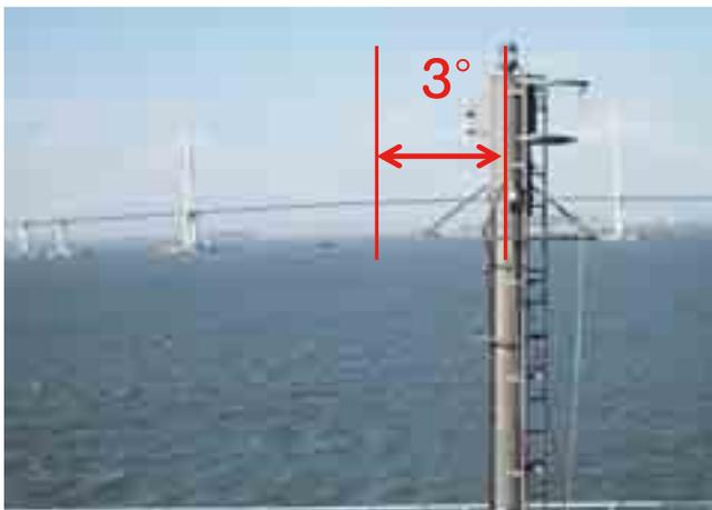
Reference photo : Leeway of 3 ° to starboard to ensure passage under center of bridge.
