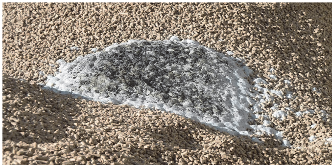
No.1 貨物上面に大量の燻蒸剤をまとめて配置し、その結果自然発熱・発火したもの。 No.1 Fumigant pellets were thrown onto the surface of the cargo in a large group and they self-heated and ignited as a consequence.
