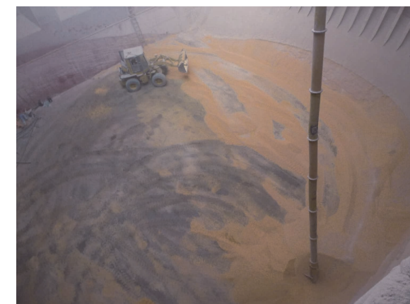
No.8 揚荷役の最終段階。ペイローダー及び空気吸引管（ニューマー）で貨物を揚げる様子。 No.8 The final stages of off-loading by use of a pay-loader and a pneumatic suction pipe.
