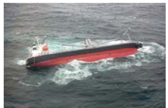
写真5 貨物の液化化が起こり、船体が左舷側に大傾斜・転覆し、後に沈没した。 Fig.5 A vessel which capsized, and later sank, because cargo on board liquefied and shifted heavily to port.
