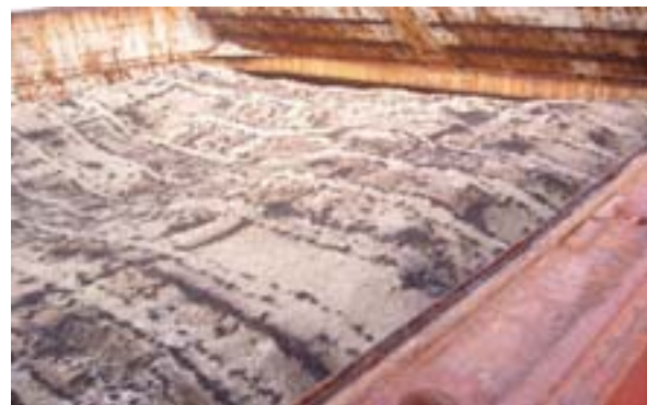
写真7 貨物表面、縦横に、ハッチカバー裏の構造部材から落下した汗の跡がみられる Fig.7 The surface of the cargo displays fore-and-aft and athwartships lines of wetting where sweat has dripped down from the stiffening members of the hatch covers.
