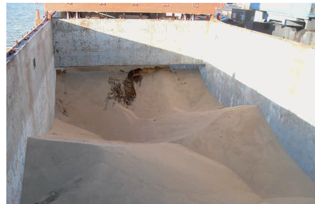
写真 16 船首端及びハッチカバー接合部に浸水による穀物の濡れ損が発生 Fig.16 The grain in this hold has been wetted by ingress at the forward end and at the sides in way of cross-joints.
