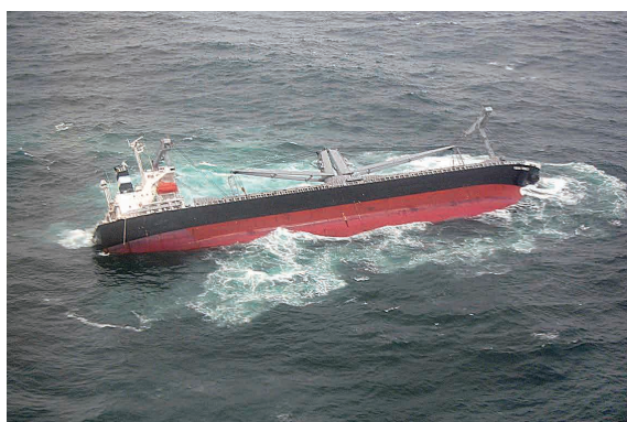
写真 5 貨物の液状化が起こり、船体が左舷側に大傾斜・転覆し、後に沈没した。 Fig.5 A vessel which capsized, and later sank, because cargo on board liquefied and shifted heavily to port.
