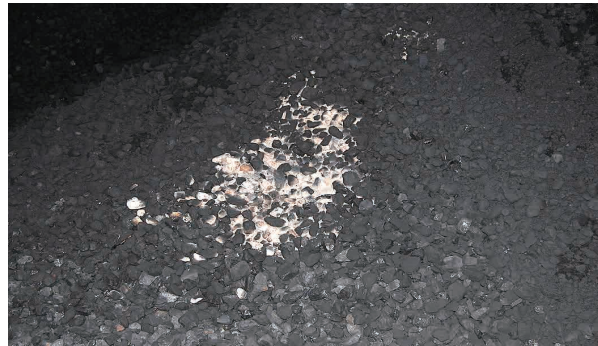
写真9 艀内で発火した石炭 Fig.9 Close-up of coal on fire in the hold.
