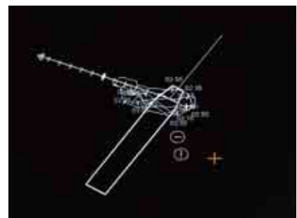
圧流走錨開始 Initiation of dragging anchor by wind pressure force
