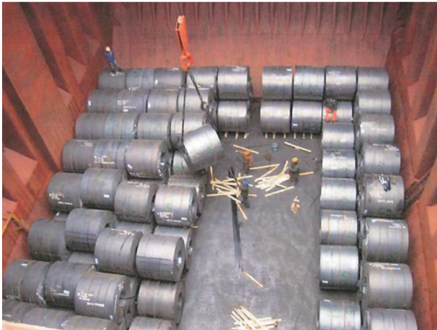
写 真 5 - 熱延コイルの積付の様子 Photo 5 - Coils of hot rolled steel sheet being loaded.
