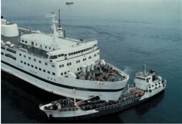
写真3 フェリーとアクリロニトリルタンカー衝突事故 Photo No.3 Collision between the car ferry and coastal tanker carrying acrylonitrile
