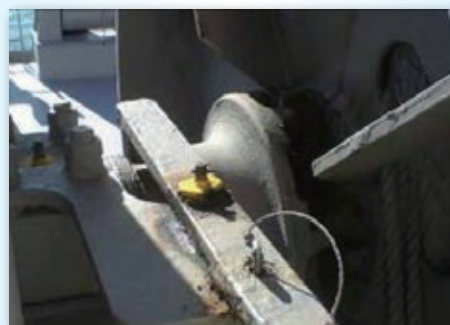
Risk of causing the operational mistake of the winch due to the clutch lever not positioned appropriately.
