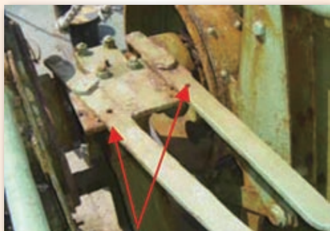
Safety pin on winch clutch lever missing.
