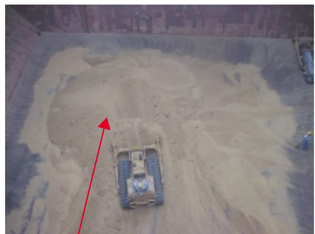
Showing gathering of the damaged cargo
