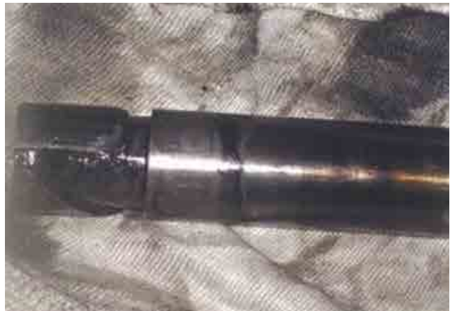
f) Wornout plunger Damage leading to speed reduction in fiscal year 2012 / reference*9
