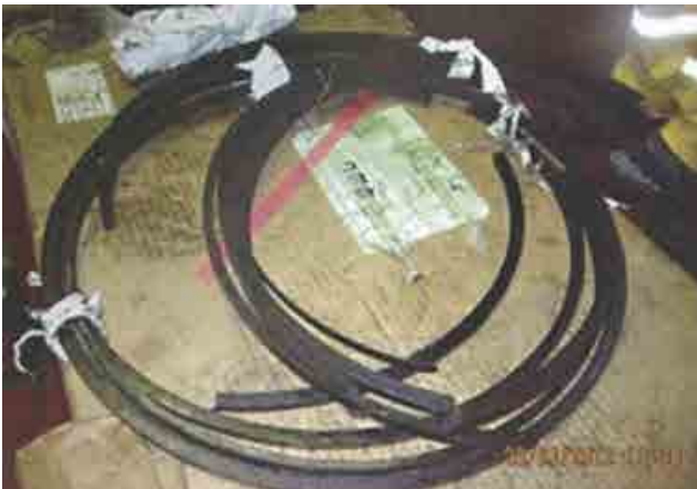
e) Broken piston ring Damage leading to speed reduction in fiscal year 2012 / reference*9
