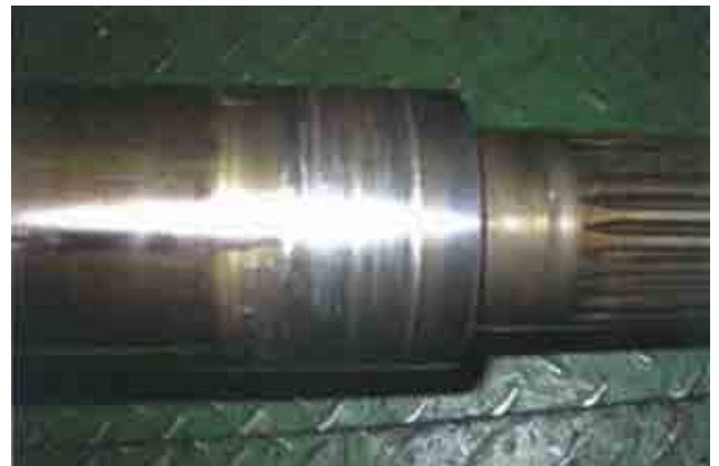
d) Scratch on turbocharger rotor shaft Damage leading to speed reduction in fiscal year 2014 / reference *4
