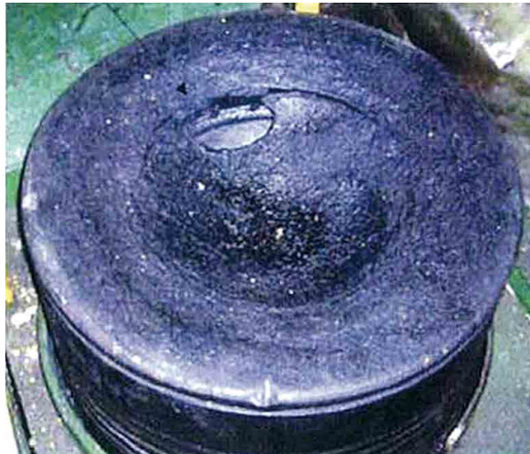
Figure 26 Hole in piston crown, damage from poor maintenance and repair mistake , requiring towing in fiscal year 2009 / reference*11
