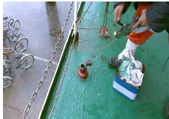
Figure 73 Measuring real tank level byTape Sounding / reference*17
