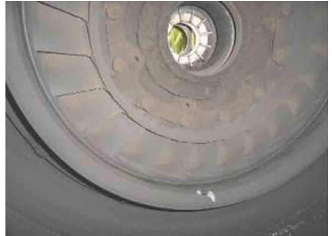
Figure 18 Excessively deformed nozzle ring / reference*7
