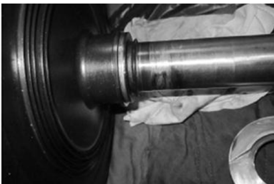
Figure 22 Scratches in rotor shaft / reference*7
