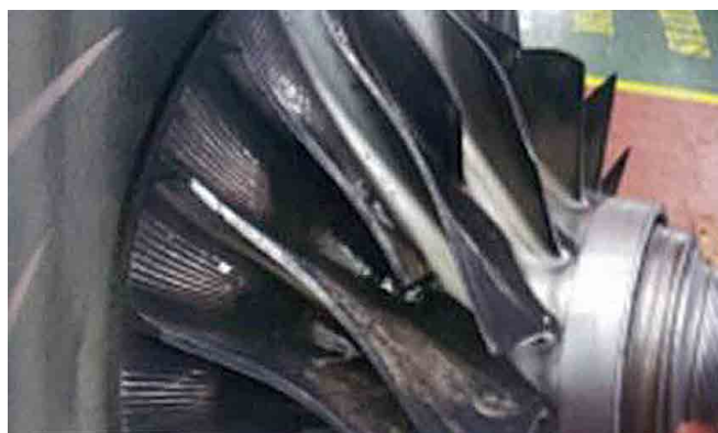
Figure 24 Scratches on compressor wheel, lubricating oil shortage damage leading to speed reduction in fiscal year 2014, reference*4
