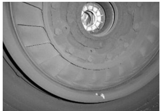
Figure 21 Carbon adhering excessively on nozzle ring / reference*7
