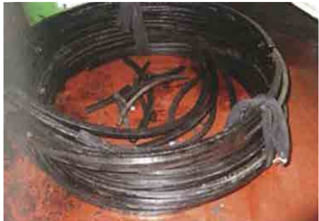
d) Broken piston ring Damage requiring towing in fiscal year 2013 / reference*8
