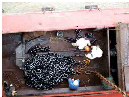
Figure 48 Connecting work of an anchor
