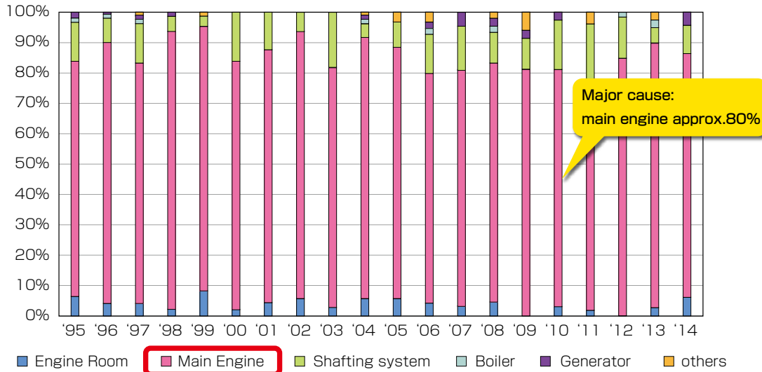
Figure 5 Percentage of machinery damage that affected ship operation /reference*4
