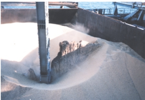
Showing damaged cargo in the top surface just under the join of the hatch cover panels (Side rolling type)
