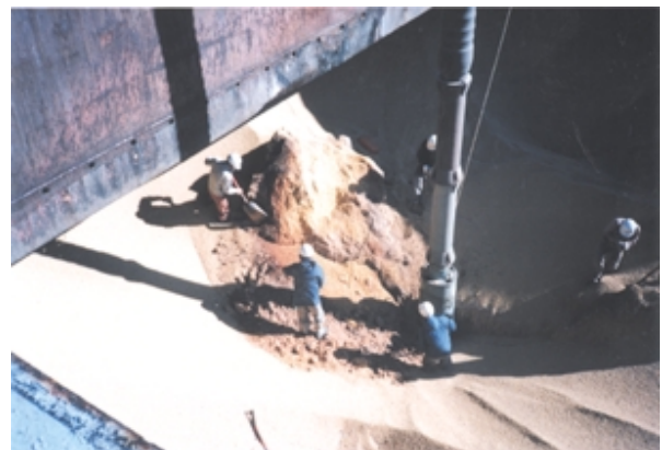
Showing the damaged cargo in the middle layer in the hold
