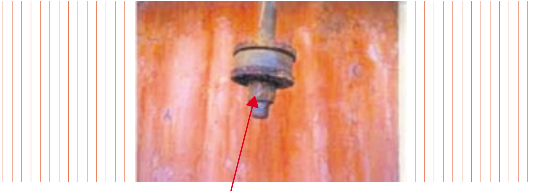
The adjusting nut frozen to the bolt
