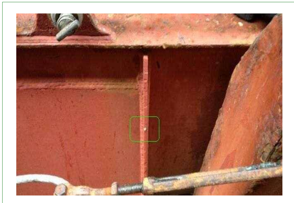
Figure 2 AGM Eggs Found Between Two Bays on a Support Beam Near a Cargo Hold Opening
