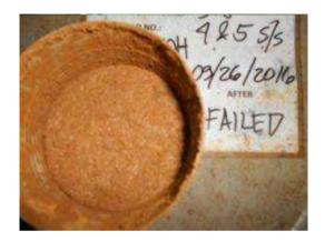
A failed test – flat pancake appearance- - FAIL carry out laboratory analysis of cargo
