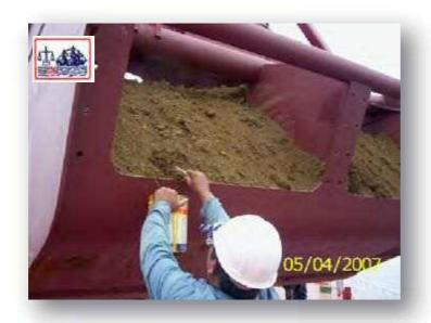
This cargo in a grab being loaded from a barge looks reasonable, however in the photo below it can be seen it failed a can test.
