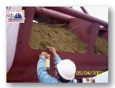
This cargo in a grab being loaded from a barge looks reasonable, however in the photo below it can be seen it failed a can test.
