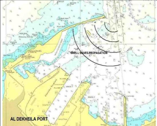
Moreover, and due to the prevailing sea currents, sea depths, Dekheila port, is characterized by high swell during rough weather, since the port entrance is facing North with a short western breakwater, while all the quays are aiming toward port entrance, where swell propagate toward the quays uninterrupted, hence, vessels berthed alongside, sometimes exercise heavy swell which may frequently cause fender damages
