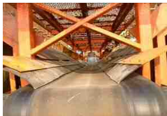
The fertilizer will drop on the conveyor belt over the iron griddle via the iron griddle
