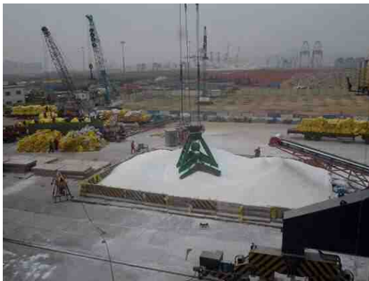
The fertilizer is being loaded on board by grab
