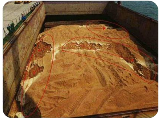
Wet damage caused by water ingress through defective hatch covers
